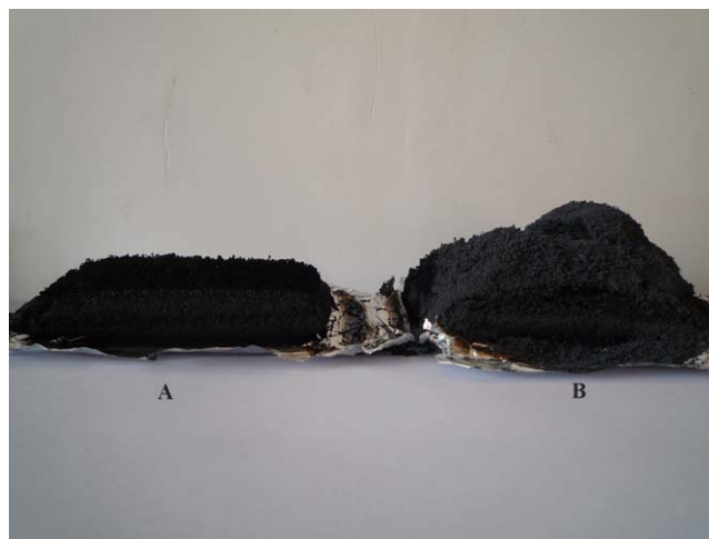
Figure 5. Photograph of the samples after CONE testing: (A) WPC/EG/APP2 and (B) WPC/EG. [Color figure can be viewed in the online issue, which is available at wileyonlinelibrary.com .]
